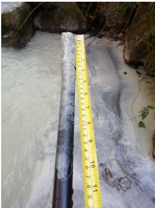
Figure 10: Kaolin-like like deposits measured as more than 15 cm deep at Piall Bridge, about 0.5 miles downstream of Quick Bridge, recorded by Julia Bertram 1430h 05Dec22
